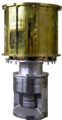
Fig. 12. The new 100 Kbar pressure cell with its He cryostat.
