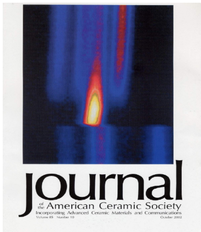
Fig. 6. The explosive SHS reaction in \text{Ti}_3\text{SiC}_2 on D20. The intermediate phase (bright spot) lasts only \sim 1 s.
